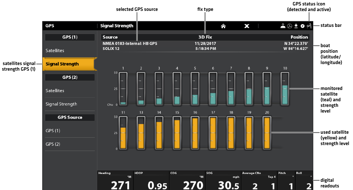
Signal Strength (GPS 1/GPS 2): displays vertical bar graphs indicating the satellite signal strengths with the respecting CNO (Carrier-to-Noise) value (0 to 60).
