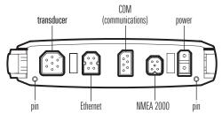
7. **Power:** Route the power cable to the main switch or fuse panel (usually located near the console). If you must connect to a battery, connect to a battery switch (not included).
