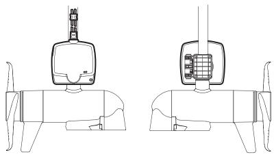
7. Fully tighten the screws until the transducer cannot be moved on the shaft. Hand-tighten only!
