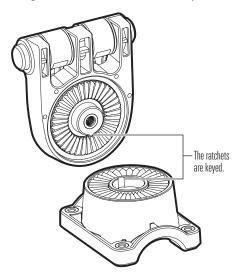
4. Secure the shaft mount with one of the included lock washers and 1/4-28 screws, using the provided hex bit. Hand tighten the screw until the lock washer is fully compressed (see the illustration *Compressing the Lock Washer*), and then tighten an additional 1/4 turn. **Hand tighten only!**
