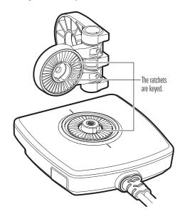
5. Secure the Landscape Mode mount to the transducer with one of the included lock washers and 1/4-28 screws, using the provided hex bit. Hand tighten the screw until the lock washer is fully compressed (see the illustration *Compressing the Lock Washer*), and then tighten an additional 1/4 turn. Hand tighten only!
