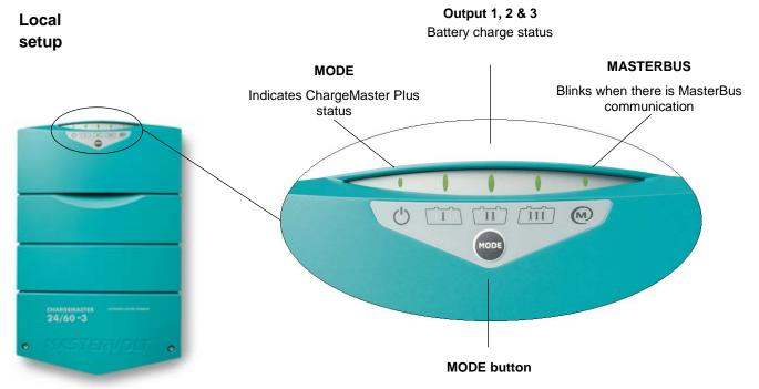
Press and hold the MODE button for 3 seconds to switch the charger on or stand-by
