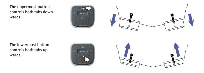
Should the trim tabs move in the wrong direction: For hydraulic trim tabs, exchange the 5 and 6 wires, for electromechanical trim tabs, reverse the wires of the actuator(s) that move in the wrong direction.
