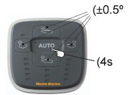
In the automatic mode, press any of the four buttons to alter the setting 0.5 degrees in a certain direction. Press more times for a greater change.
