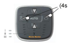
Press the left and right button simultaneously for 4 seconds until an indicator in the middle starts to blink.
