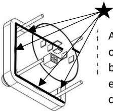
Apply a bead of silicone sealant around the underside of the display where the rubber overlay meets the black potting material. This will prevent water from entering under the display and reaching the wiring connections.
