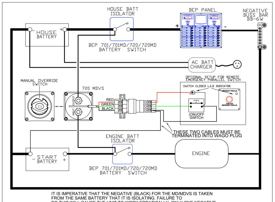
DO THIS WILL CAUSE THE UNIT TO WORK ERRATICALLY. ONLY ONE NEGATIVE MUST BE SUPPLIED TO EACH UNIT FOR CORRECT OPERATION.
