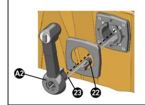
2 Position lever unit. Cable guide (24) shall be opposite to lever in neutral position. Make the cable pass through the flange opening (3) that is as close as possible to item (24). Attach control lever using screw (M) and press on cap (N).
