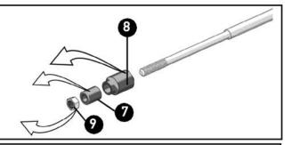
2 Insert the cable into the (black) connector (G) and fasten it with the split pin (I).
