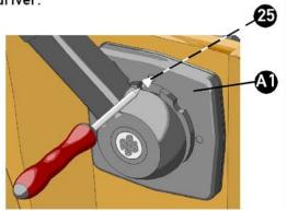
Adjust throttle lever friction turning on screw (25) with a Phillips head screwdriver (clockwise to increase and counterclockwise to decrease the friction). When adjustment is ended, close the drilled hole by inserting the provided screw cover (P)
