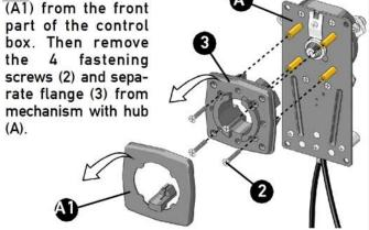
Fix flange (3) using screws (B), washers (D), nuts (C). The flange should be positioned in such a way that the slit (x) is aligned with sliding the element in the control lever that provides the locking in neutral.
