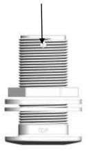
TruDesign brand is printed on the nut. This enables clear identification that genuine fittings are installed.
