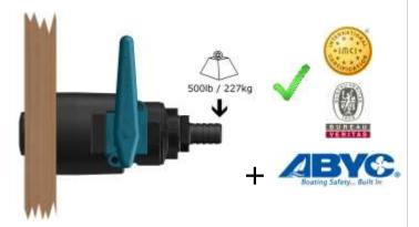
In accordance with ISO 9093-2 standards, Skin Fittings (Thru Hulls) are subjected to a 155kg (341.7lb) load, applied to the threaded section for a minimum of 30 seconds, without any damage occurring. TruDesign Skin Fittings (Thru Hulls) meet this standard.
