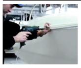
The track, in PVC rigid is very elastic can be cold fitted and it follows perfectly the bends of the boat except very acute bending radius (also only 8/10 cm – see tab.)
