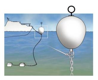
Do not expose the buoy to a load of more than 60% of its total buoyancy. Please also consider additional weight/load caused by marine growth, currents, wind and waves.
