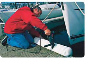
The Bumper can be secured with screws on the pontoon.
