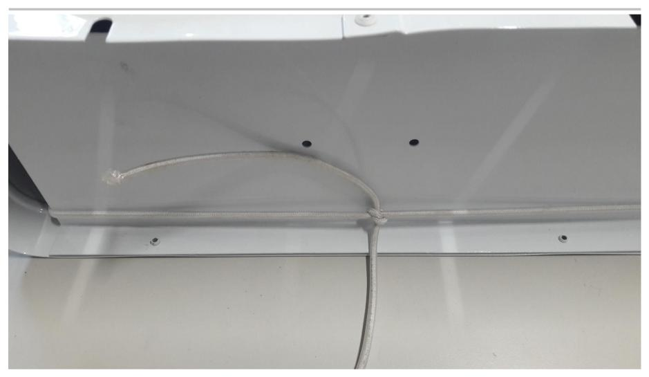
Pull the rubber band until and reach a good tension. This should be enough to let the door open and close properly. A few tries are expected. Tight the knot.
