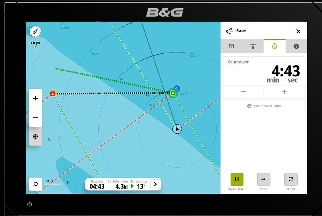
Race Mode enabled: showing start line with laylines, line bias, range-rings and Race Timer controls
