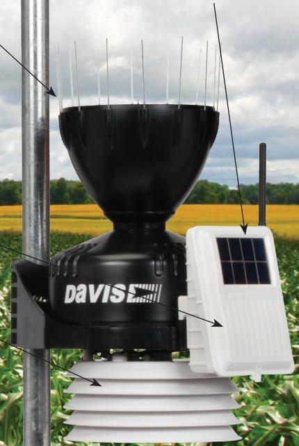
Weather-resistant shelter houses electronic components for added protection against the elements.
