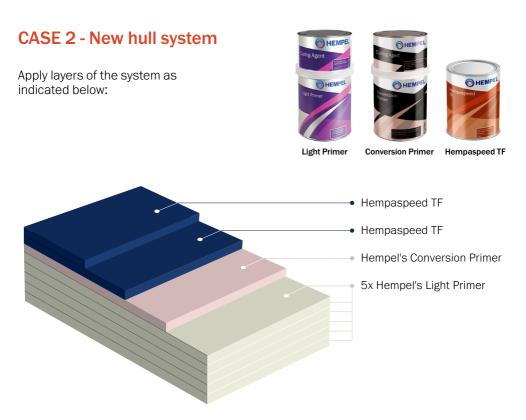
For a full season protection, the substrate needs to be sealed with Hempel's Light Primer (300µm dft) before applying Hempel's Conversion Primer and 2 coats of Hempaspeed TF. Follow stated overcoating intervals between the primer and product to ensure intercoat adhesion.
