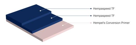
For full season protection - no need to remove old coating, just 1 coat of Hempel's Conversion Primer needs to be applied before applying 2 coats of Hempaspeed TF.
