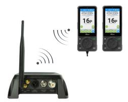
Both Cortex H1 and Cortex H1P handsets connect to the Hub using Wifi and only needs power to the Bulkhead Connector or Charging
