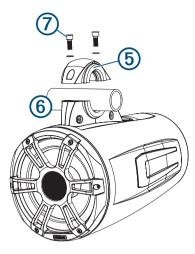
**14** Attach the top of the bracket to the base of the bracket using the included screws ⑦ with a 6 mm hex driver or hex key.
