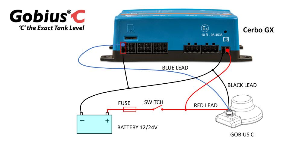
Connect Gobius C red lead to battery plus (after switch) and to Cerbo GX "Power+" Connect Gobius C black lead to battery minus, to Cerbo GX Tank1 "GND" and to Cerbo GX "Power-" Connect Gobius C blue lead to Cerbo GX Tank1 "DATA"
