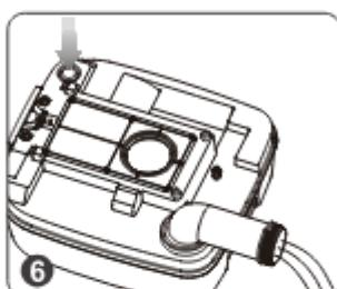
Press and hold the exhaust button and drain again
