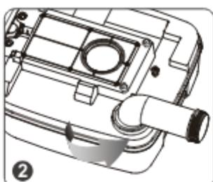
Turn out the drain pipe and open the drain pipe cover
