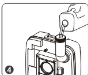
Lift the waste water tank and add 1-2L of clean water
