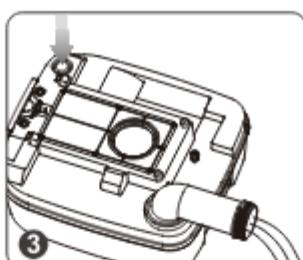
Press the exhaust button and discharge the sewage
