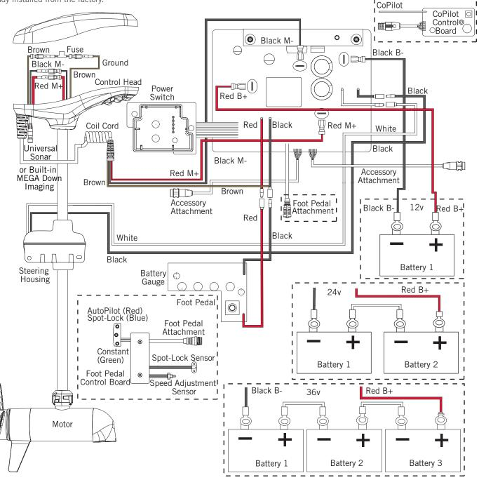
**NOTICE:** This is a multi-voltage diagram. Double-check your motor's voltage for proper connections. Over-Current Protection Devices are not shown in this illustration. If equipped with Universal Sonar or Built-in MEGA Down Imaging, please visit the website at minnkotamotors.com for additional information.
