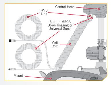
**NOTICE:** Critical cable routing for 60" and 72" motors with i-Pilot Link and Built-in MEGA Down Imaging. Accessory Cables must exit the Coil Cord leaving three or more open coils between where the cables exit and the motor base; as assembled by the factory. Routing the cables in any other manner will not allow the motor to stow properly.
