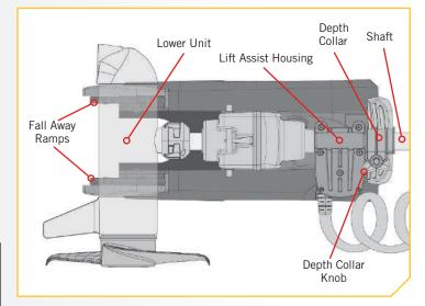
**NOTICE:** Slide the Depth Collar down and secure it against the top of the Steering Housing when stowed to secure the motor in place and prevent accidental deployment.
