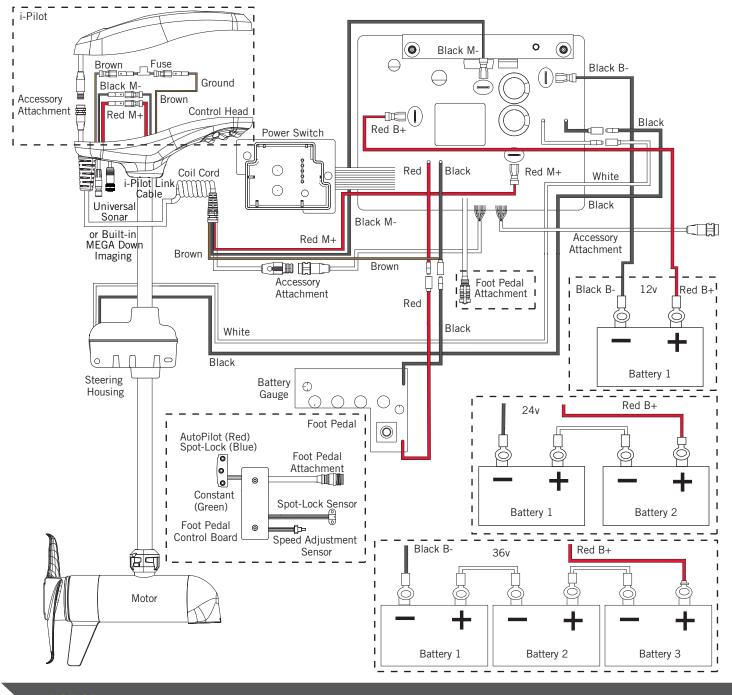
**NOTICE:** This is a multi-voltage diagram. Double-check your motor's voltage for proper connections. Over-Current Protection Devices are not shown in this illustration. If equipped with Universal Sonar or Built-in MEGA Down Imaging, please visit the website at minnkotamotors.com for additional information.
