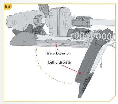
9 o. Replace the four sideplate screws using a #3 or #2 Phillips screwdriver. Two of these screws will be located on each side of the mount.
