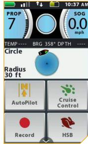
The Circle Mode Active band appears when the navigation is set to Circle Mode. The current circle radius is set to 30 feet.
