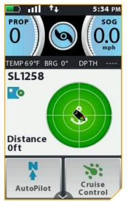
The Spot-Lock Active Band appears when Spot-Lock is engaged. The Save icon indicates that the Spot-Lock has not yet been saved.
