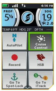
The Home Screen Buttons are Active and the Cruise Control button has been selected using the Screen Navigation 8 button and then the Ok button.
