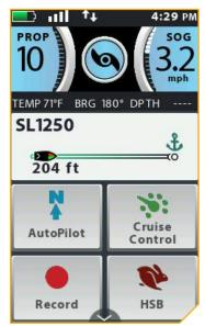
The Go To Spot-Lock Active Band appears when the boat is navigating to a saved Spot-Lock. The Spot-Lock being navigated to is 204 feet away.
