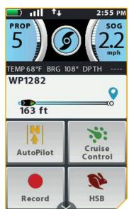
The Go To Waypoint Active Band appears when the boat is navigating to a saved Waypoint. The Waypoint 1282 is 163 feet away.
