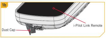
Plug the USB Remote Charger into the remote. The Charging Indicator Light will illuminate whenever an energized charging cable is connected.
