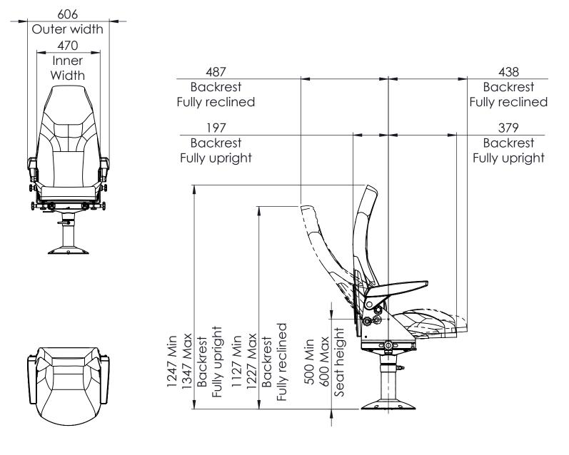
All sitting heights measured without load - a variation may occur depending on the load due to contraction of gas-struts, springs, upholstery and third part equipment.
