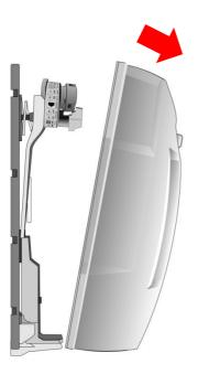
5. Bend the antenna backwards and retain it in the recess to left or right.
