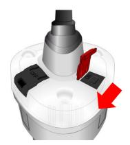
The strobe light will start to flash immediately; however, the EPIRB will not make any distress transmissions for approximately 50 seconds. This allows time to turn off the EPIRB if it has been activated accidentally. When the green indicator starts to flash, distress transmissions have started.
