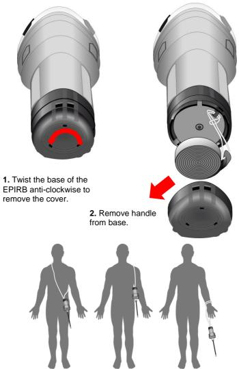
**3.** Adjust the carry handle to secure the EPIRB across the body, around a shoulder, arm or wrist during emergency evacuation prior to activation.
