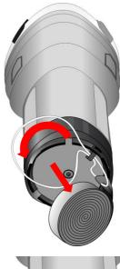
**5.** Using a 4mm hex key, unscrew retaining bolt until loose. Do not remove at this stage.
