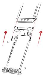
Slide stylus into the top brackets from the side. **Do not snap the stylus into place from the top.**
