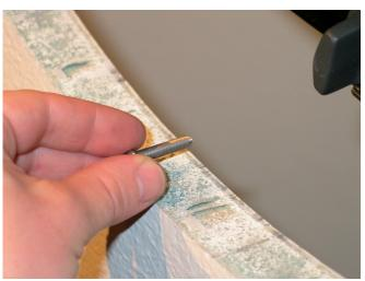
5. Mount the portlight and the innerframe on the hull by fastening the bolts. Apply a lubricant on the bolts and the maximum torque is 2,5 Nm.
