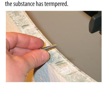
5a. Mount the portlight and the inner trim on the hull by fastening the bolts.
