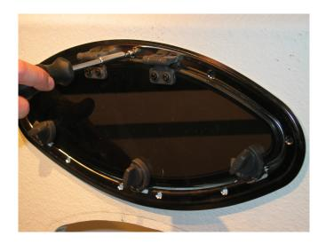
5c. Apply a lubricant on the bolts and the maximum torque is 2,5 Nm.
