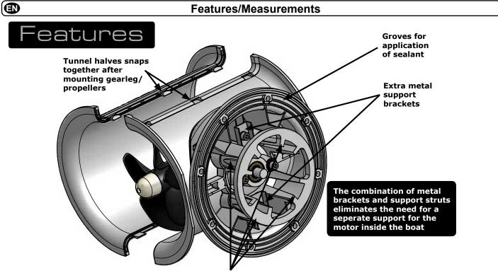
Integrated support struts for each of the 4 motor bracket legs
