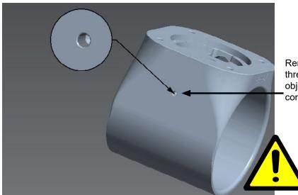
Remove galvanic corrotion from the threaded hole with a drill bit or sharp object to establish proper electrical connection.
