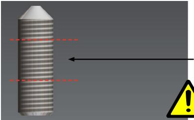
Secure the bolt by using Locktite (LocTite #2701 or similar) on the middle section of the bolt.
