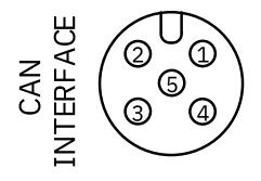
M12 Input Male Connector (View into connector) Pin 1 NC Pin 2 NC Pin 3 GND Pin 4 CAN-H Pin 5 CAN-L
