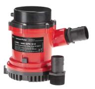
The SPX Johnson Pump Marine submersible pumps can handle most bilge pump applications. Heavy duty motors with stainless steel (SS2343) shaft and tough thermoplastic bodies provide for a long pump life. With an automatic switch installed, the pump automatically starts on when there is water in the bilge and shuts off when it is dry. Salt water tested - salt water tough.
