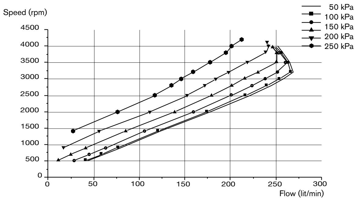
All performance curves are based on water at 20°C (68°F) and full cam.
