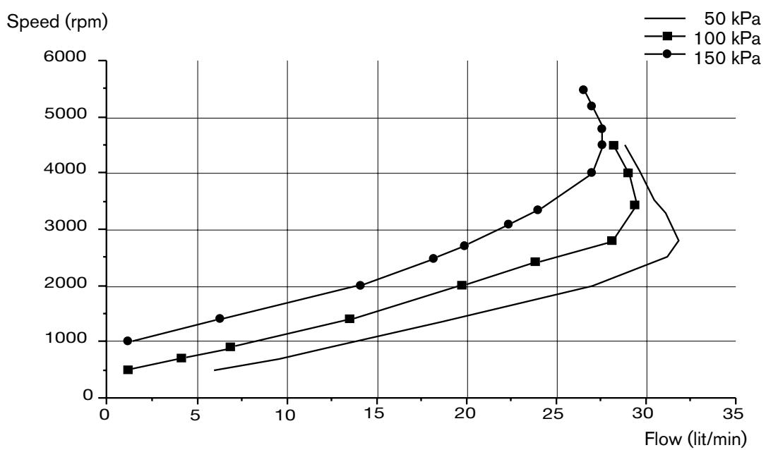
All performance curves are based on water at 20°C (68°F) and full cam.
