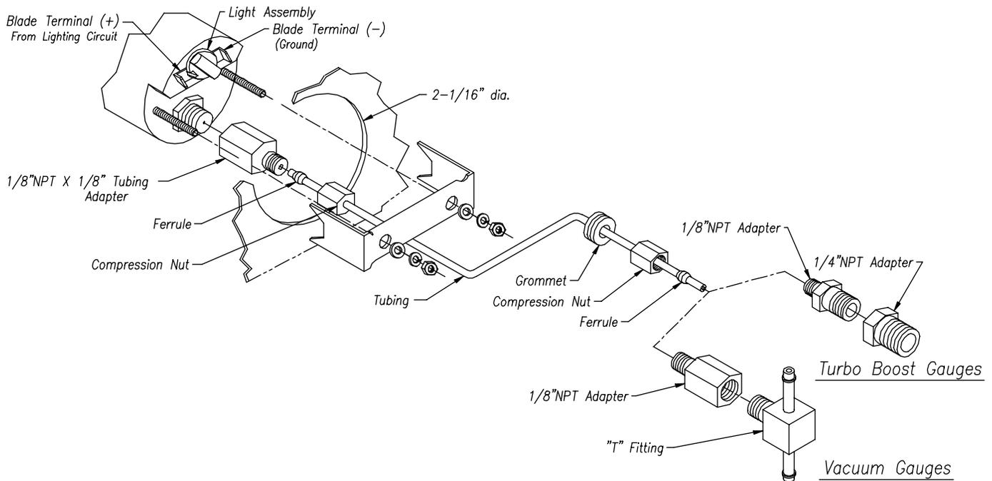
**CAUTION:** Disconnect the battery during installation. Tighten nuts on the back clamp only slightly more than you can tighten with your fingers. Six **inch-pounds** of torque is sufficient. Over tightening may result in damage to the instrument and may void your warranty.
