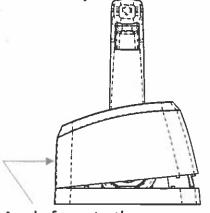
Apply force to the rearward face of the bezel until Tab 2 disengages
