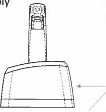
Apply force to the forward face of the bezel until Tab 1 disengages
