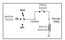
**STEP 1.** With the Control in NEUTRAL, connect one wire of the tester to the common terminal, and one wire to the "NO" (Normally Open) Terminal. The test light MUST light.
