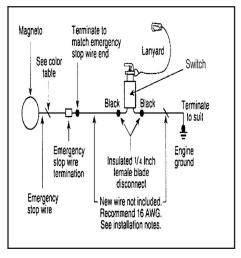
Diagram B. Outboard Wiring.
