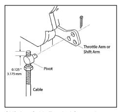
Shift Arm Cable Terminal Connection for 3300/33C Cable.
