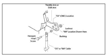
Shift Arm Cable Terminal Connection for "OS" is BRP/OMC/Johnson and Evinrude. "KM" is Mercury, MerCruiser.
