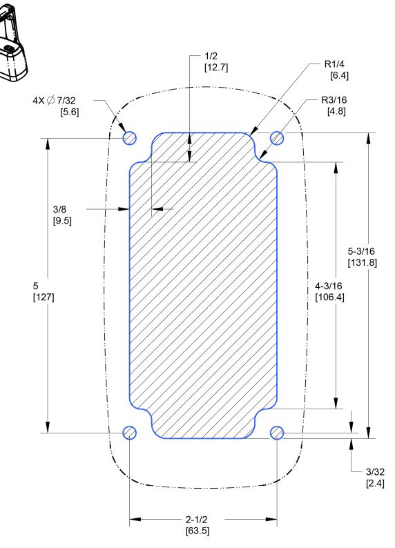
REMOVE ENTIRE HATCHED AREA AND DRILL FOUR 7/32 [5.6] DIAMETER HOLES.
