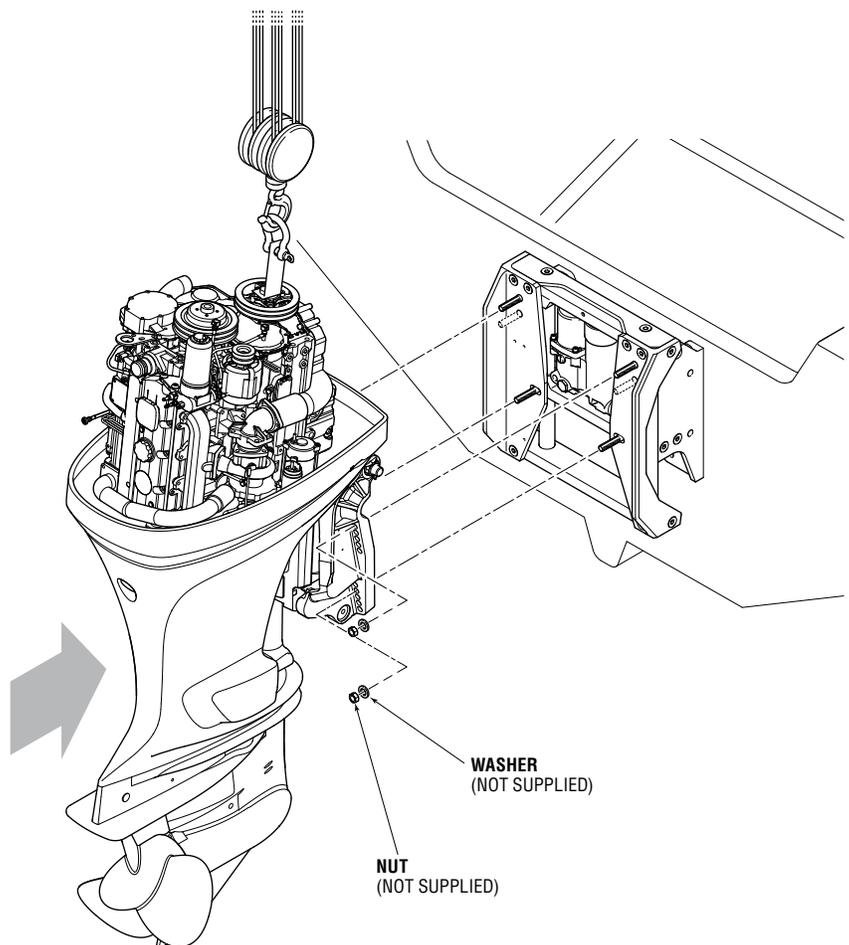
Figure 14. Outboard installation.
