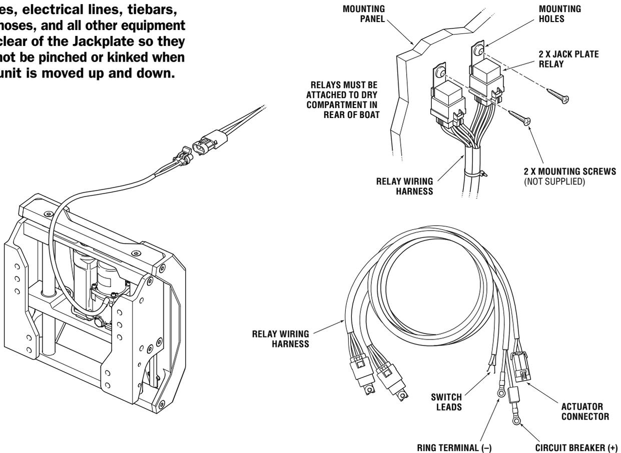
Figure 9. Relay Wiring Harness installation and connections.
